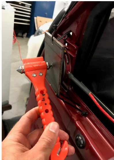
Figure 13: Load cell and hammer used for measurement of impact force. Image Source: AAA
