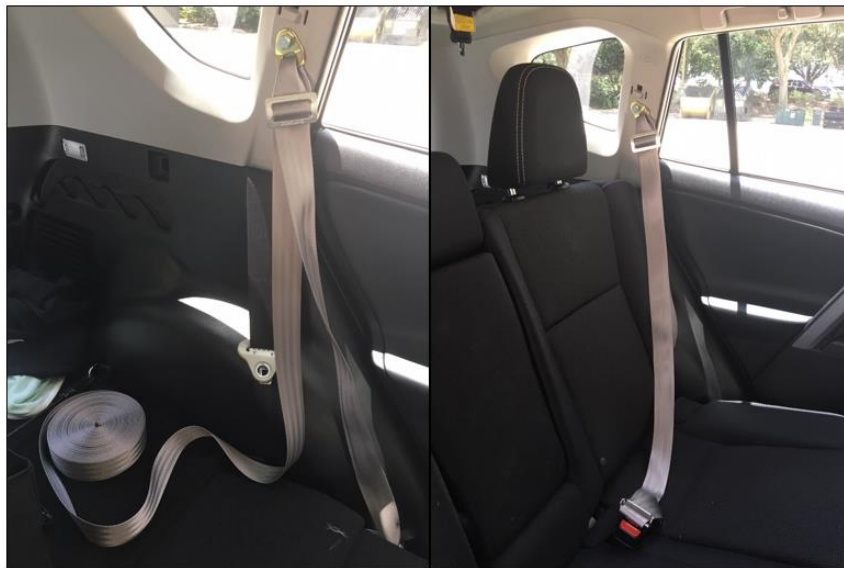
Figure 9: Setup for seat belt-cutting test. Image Source: AAA
