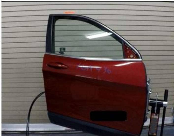
Figure 11: Setup for window-break testing. Image Source: AAA
