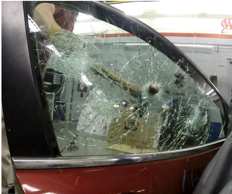
Figure 18: Attempt to break laminated window with ball-peen hammer. Image Source: AAA
