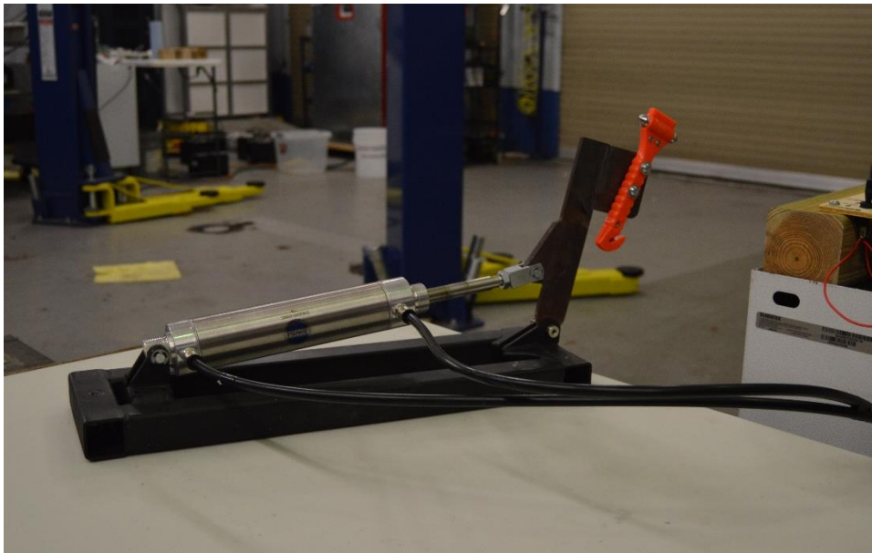
Figure 12: Pneumatic arm for hammer tool testing. Image Source: AAA
