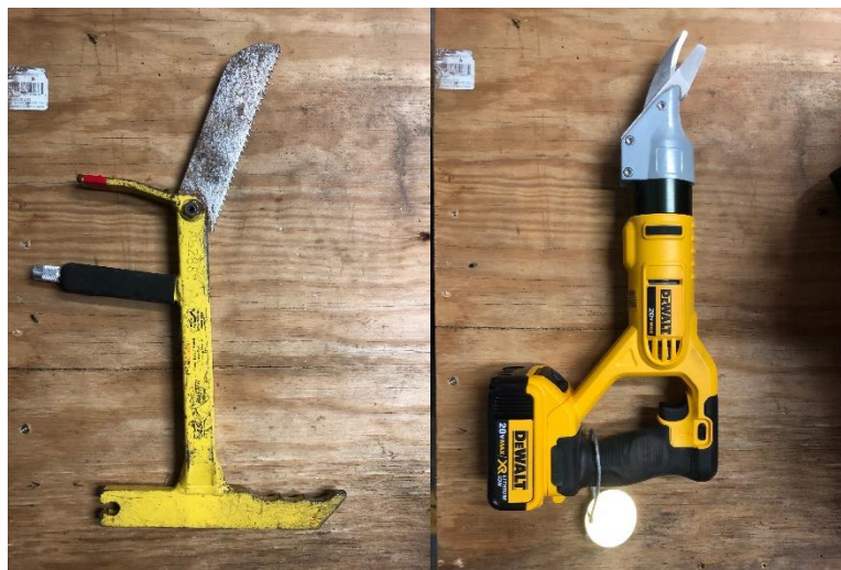
Figure 19: Examples of professional glass removal tools. Image Source: Orange County Fire and Rescue
